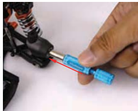
2. Insert the Bearing Remover into the bearing.
