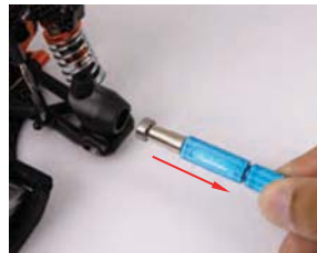
4. Pull out the Bearing Remover.
