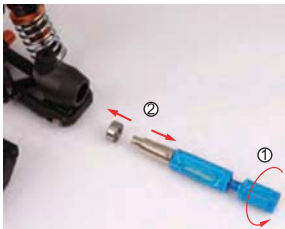
5. Unscrew the handscrew then pull out the bearing.
