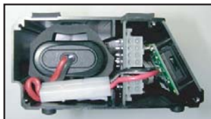
4. Insert your battery pack into the CTX-D carefully and connect battery connector to female Tamiya connector inside.
