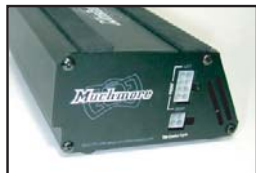
5. Place left side plate properly, then tighten 4 screws gently. Make sure battery wires do not bend.
